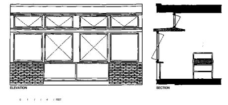
Figure 21 Elevation and section of the windows in the experimental wards at Larkjield Hospital
