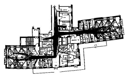
Figure 9 String diagram showing the pattern of movement of a nurse during a complete tour of duty
