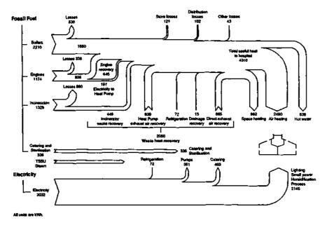
Figure 25 Low Energy Hospital schematic of energy flows
