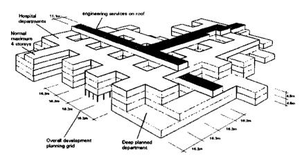
Figure 16 Diagram of a Harness Hospital System
