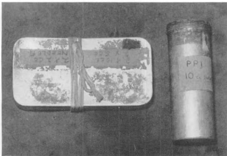
Syringes enclosed in tin containers. Steam will be unable to penetrate the containers
